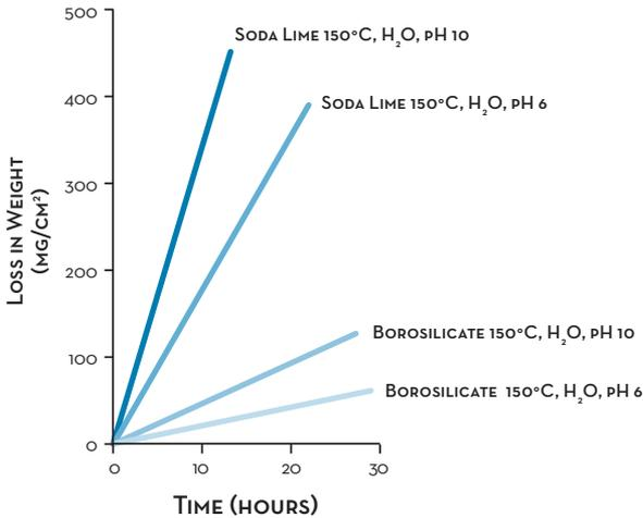
In investigating for chemically induced disintegration of Soda Lime and Borosilicate Glass, it was found that Borosilicate was much more resistant. This occurred not only at slightly acidic conditions (pH 6), but also when the pH was raised to a value of 10 (alkaline). As shown on the chart, the degradation of Soda Lime glass is 10 times greater than that of Borosilicate glass. This considerable divergence in resistance properties begins at 134°C, the initial temperature in the study.
