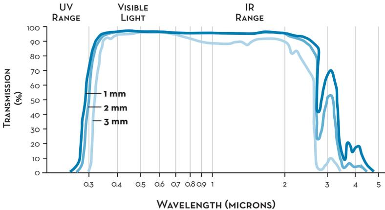
**SODA LIME GLASS** owes its popularity to the fact that it is the least expensive and most common type of glass. Soda lime glass is used in the manufacture of bottles, light bulbs and windows. It is comprised of silica, soda, lime, magnesia and alumina.
