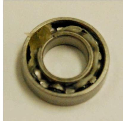
*A wax or flux substance along with a filter fiber thread was lodged in the bearing during initial start-up.*
